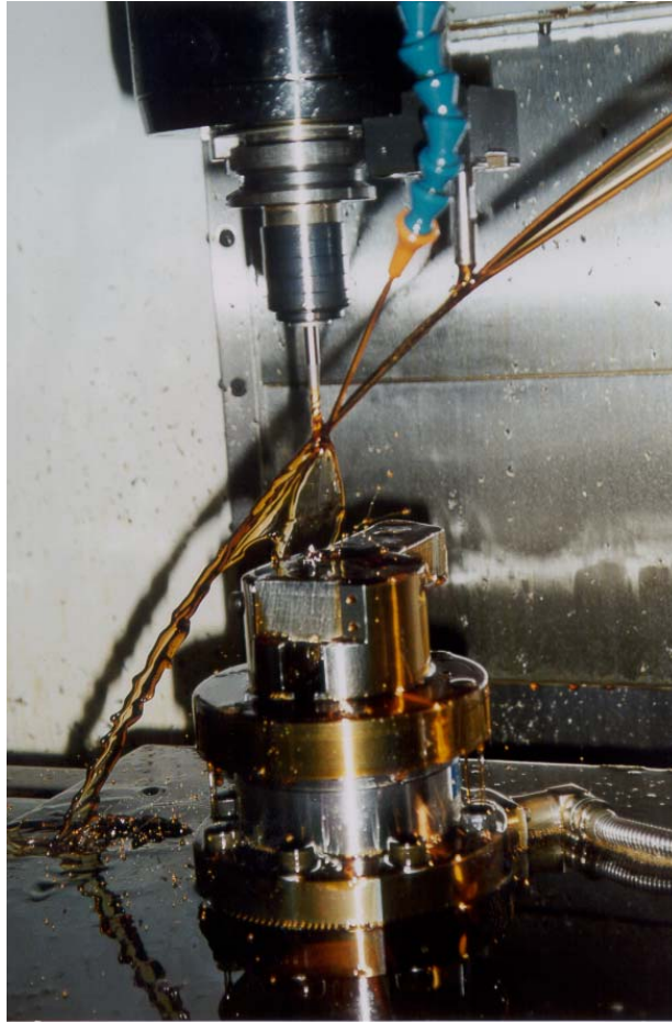
Figure 4.4. A photograph of the Kistler dynamometer set-up in the HAAS CNC machining centre, showing an M6 spiral flute tap mounted in a non-synchronous (floating) attachment with lubricant directed at the tap flutes.
